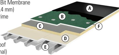
*Modified bitumen without base sheet. Mod Bit is torched or set in hot asphalt. BUR is minimum 3-ply.*
