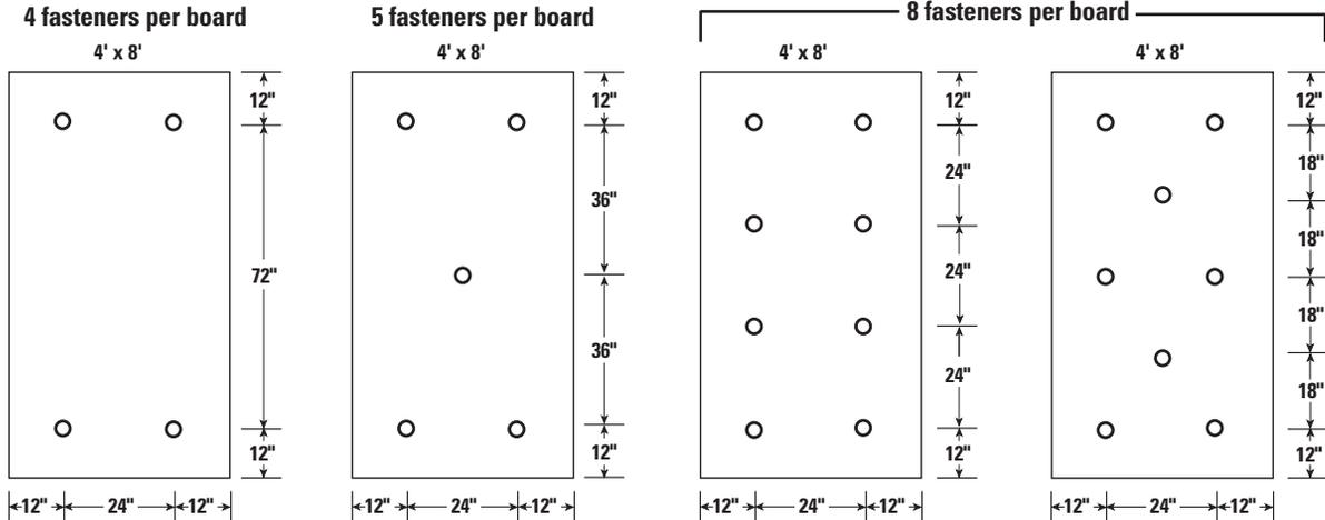
Note: Preliminary insulation or mechanically attached roof covering requires a minimum of 4 fasteners per 4' x 8' board in FM assemblies.
