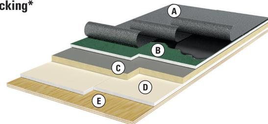
*\*Note: The UL 790 classification for DensDeck provides that the use of DensDeck roof boards as a barrier board over a combustible deck permits the use of any classified roofing system which would otherwise be limited to use over a noncombustible deck. When used, the insulation must consist of one of the types specified. For additional information, consult the UL certifications directory under category TGFU (Roofing Systems).*
