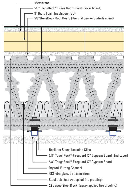
Tests per ASTM E90 and ASTM E413, were conducted in 2011 at Riverbank Acoustical Laboratories. Results are based on characteristics, properties and performance of materials and systems obtained under controlled test conditions. Actual results may vary and Georgia-Pacific makes no representations or warranties concerning the STC rating of any assembly.
