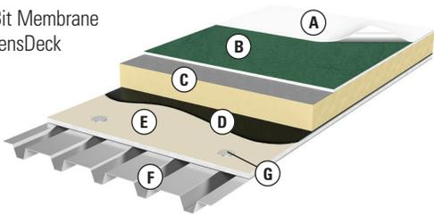
DensDeck Roof Board (1/2" (12.7 mm) or 5/8" (15.9 mm)) and fully adhered single ply membranes FM-rated 60 PSF with insulation attached with asphalt adhesive.
